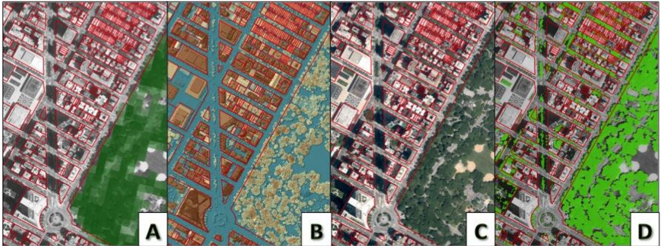
Figure 2. Tree canopy comparison between the 30m National Land Cover Database (NLCD) and the 1m land cover proposed for this study. NLCD fails to capture individual trees and small forested patches and the pixels cross property parcel boundaries (red lines). Lidar data is unaffected by shadows, allowing for more accurate mapping, particularly in urban areas and locations with high topographic relief (B). When the Lidar data is combined with high-resolution imagery (C) tree canopy can be mapped with such accuracy, than even young street trees in building shadows can be mapped (D).
